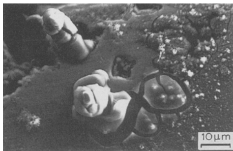
Fig. 3. Pitting corrosion in alloy HC after a 18 h exposure in air-saturated 0.1 M NaCl.
